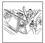
The remote negative (–) terminal is located in the front of the engine compartment, near the engine oil dipstick.
